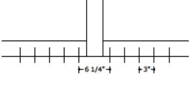
CONDITION 2 HEAD/SILL WITHOUT SUB BUCK (3/4" MAX SHIM)
